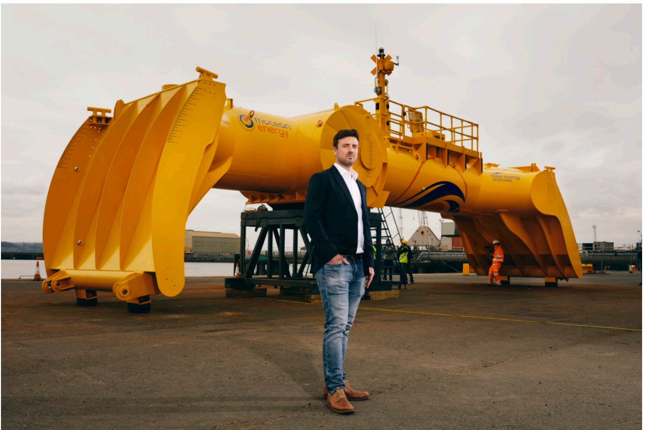
Mocean Energy's Managing Director Cameron McNatt with Mocean Energy's Blue X wave energy converter at Forth Ports' Rosyth Docks.
