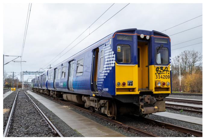
Exterior view of a 314 Class electric train sitting at the Scotrail Yoker Depot in Yoker, Glasgow on 14th December 2020. The train has been decommissioned and will be taken to Bo'ness where it will be converted to run on hydrogen.
