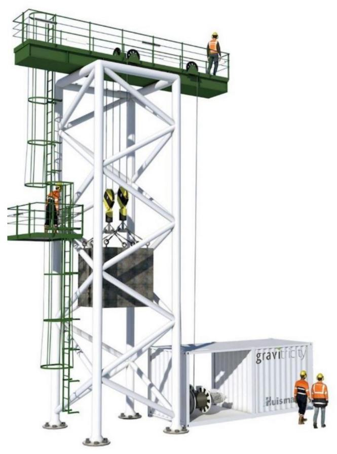
Gravitricity Concept Demonstrator Gravitricity uses one or more heavy weights suspended in a deep shaft by cables attached to winches. When there is excess
