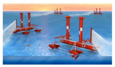
An artist's impression of hydrofoil geny vessels in action for Lathan's proposal to reverse global warming with marine cloud brightening. Propulsion comes from Fettner rotors. Energy generation comes from alternating pitch-wariation of hydrofoils driving parallelogram linkages to habitatile green. Efficient works to generate dreams, alternation generated and habitatile green green and green and proposal physicisms proposal to the proposal proposal proposal dreams.
