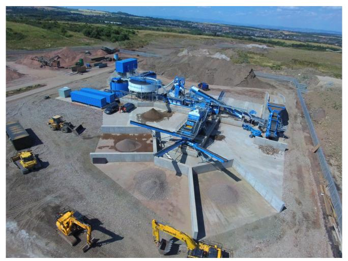
Large scale investment in new recycling facility Investment in the £3.8m recycling centre includes a £2.1m spend on high efficiency CDE equipment, with a capacity to recycle 400,000 tonnes of construction, demolition and excavation waste per year.
