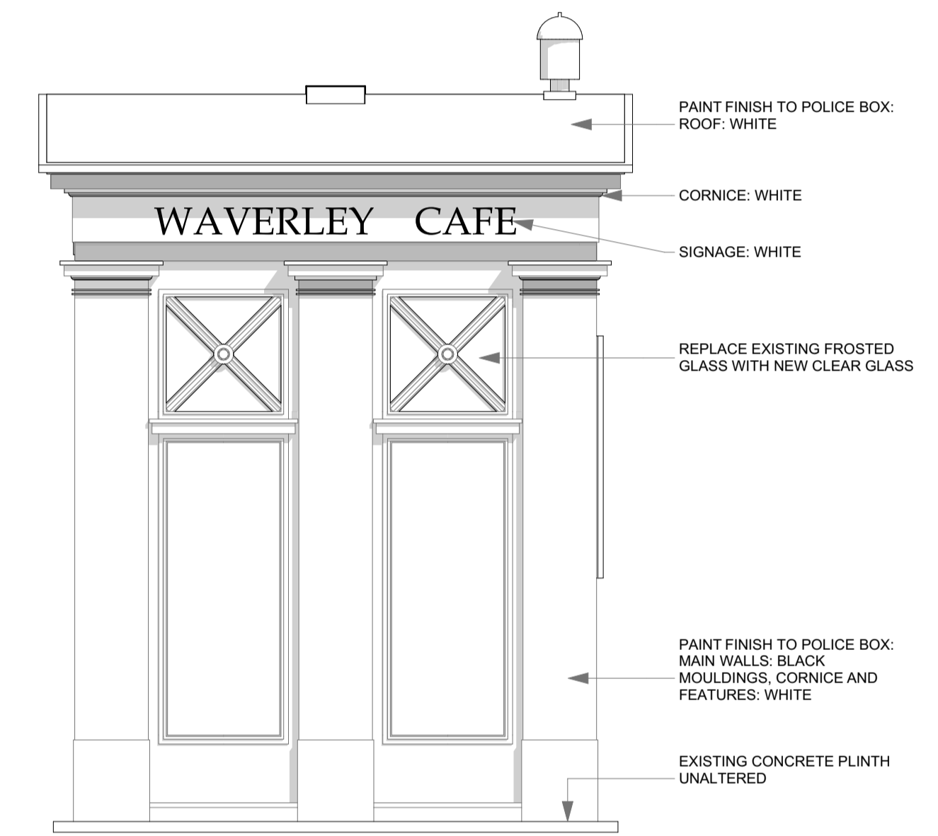
Proposed North Elevation 1:20
